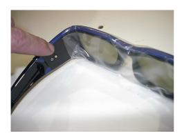
To activate the 3D glasses simply press the activation button in inside of the left temple with the glasses pointing towards your 3D television or 3D transmitter. To turn them off simply put the glasses back inside of the 3D glasses cleaning/storage case.
